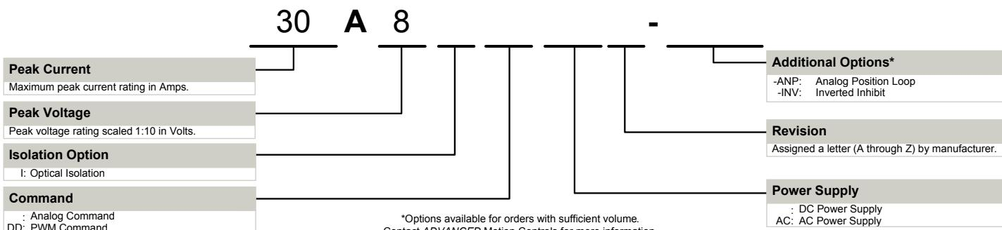
ADVANCED Motion Controls analog series of servo drives are available in many configurations. Note that not all possible part number combinations are offered as standard drives. All models listed in the selection tables of the website are readily available, standard product offerings.
